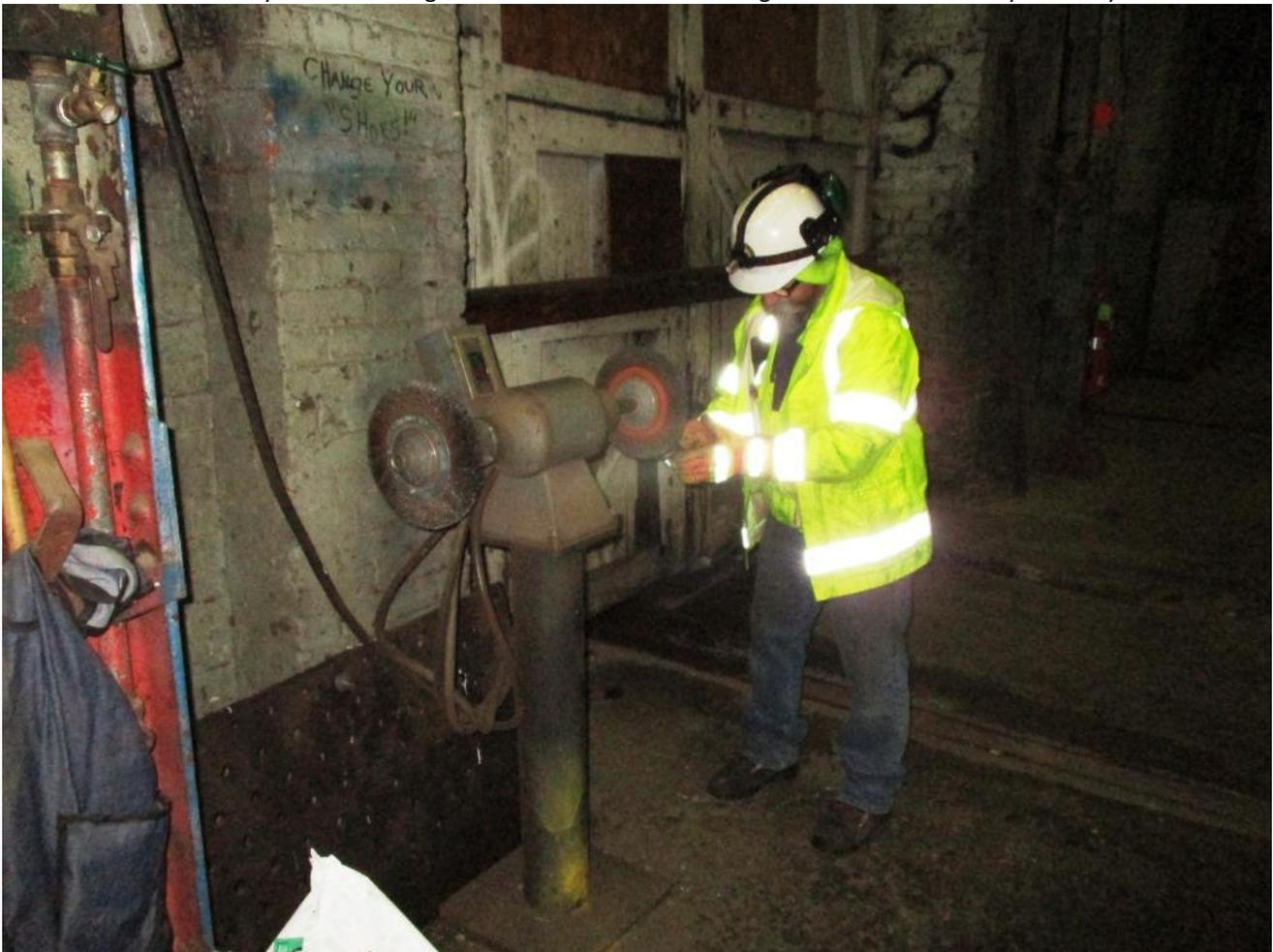
Joe uses the wire brush to clean up the bolts that attach the 125's hydraulic cylinder to its base
