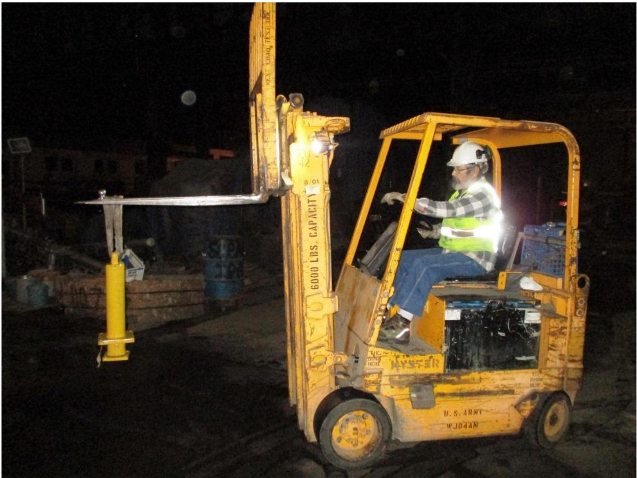
Ed K. uses the Hyster forklift to grab the Jackson 125 tie-exchanger's rebuilt turntable hydraulic cylinder
