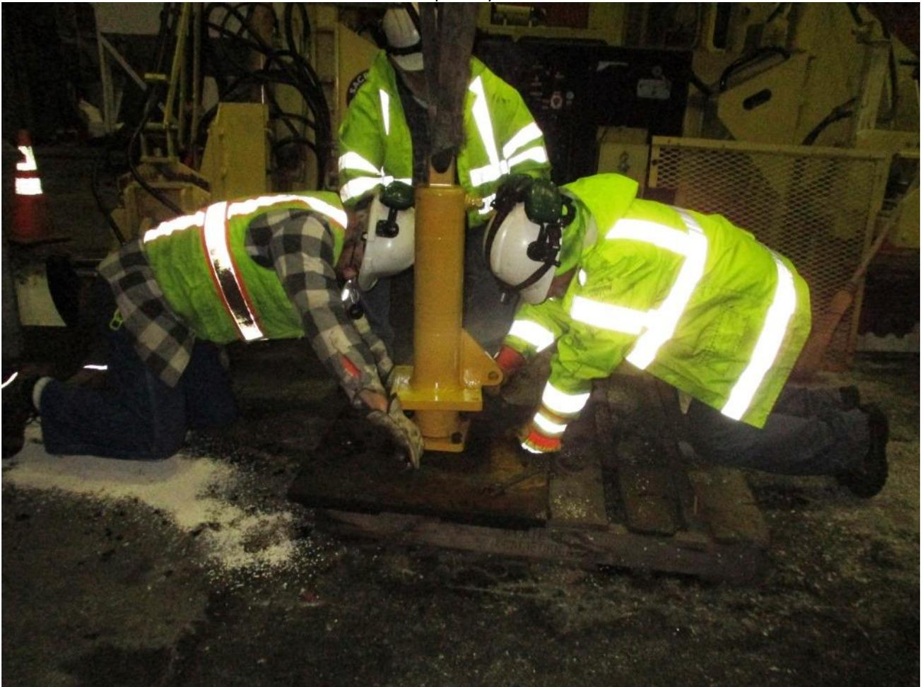
Ed K., Frank, and Joe bolt the 125's turntable hydraulic cylinder to its base
