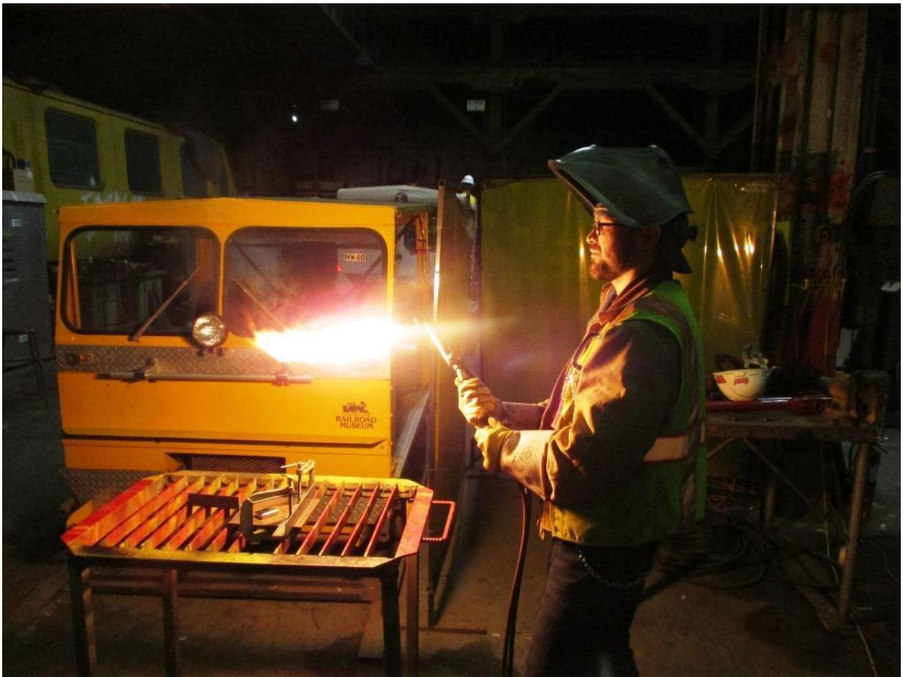
Kyle fires-up his cutting torch as he fabricates new draw-bar connectors for the hopper cars
